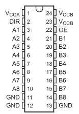
Figure 5-1. DB, DGV, or PW Packages, 24-Pin SSOP, TVSOP, or TSSOP (Top View)
