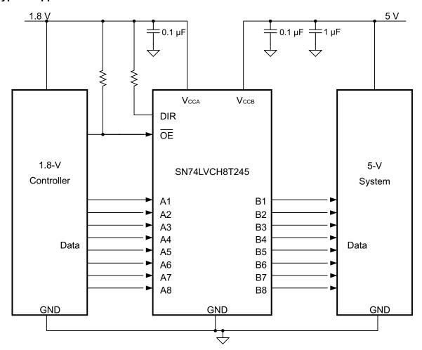
Figure 9-1. Typical Application Circuit
