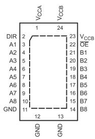
Figure 5-2. RHL Package, 24-Pin VQFN (Top View)
