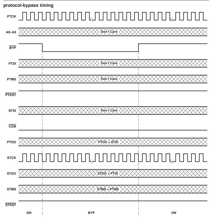
Figure 19. Protocol-Bypass Timing, Prior Connect Status = ON
