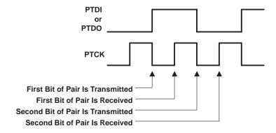
Figure 3. Bit-Pair Timing (Data Zero Shown)
