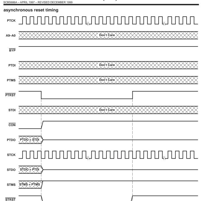
Figure 21. Asynchronous Reset Timing, Prior Connect Status = ON
