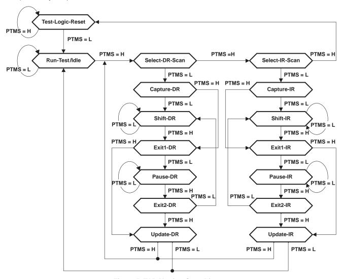
Figure 5. TAP-Monitor State Diagram
