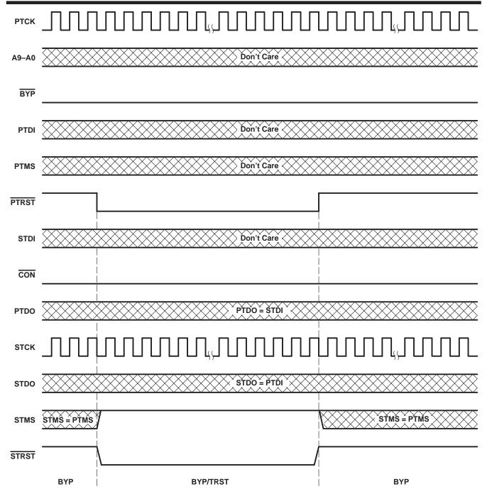
Figure 23. Asynchronous Reset Timing,  $\overline{BYP} = L$
