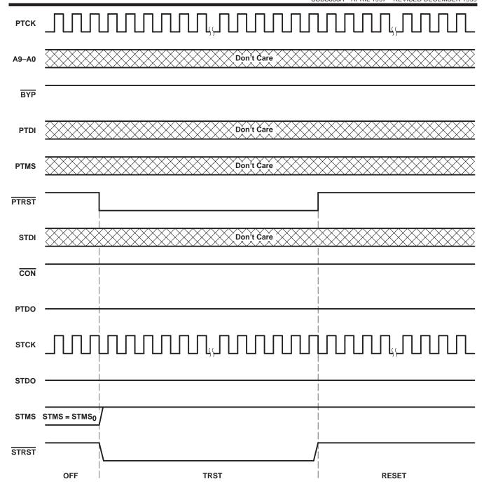
Figure 22. Asynchronous Reset Timing, Prior Connect Status = OFF
