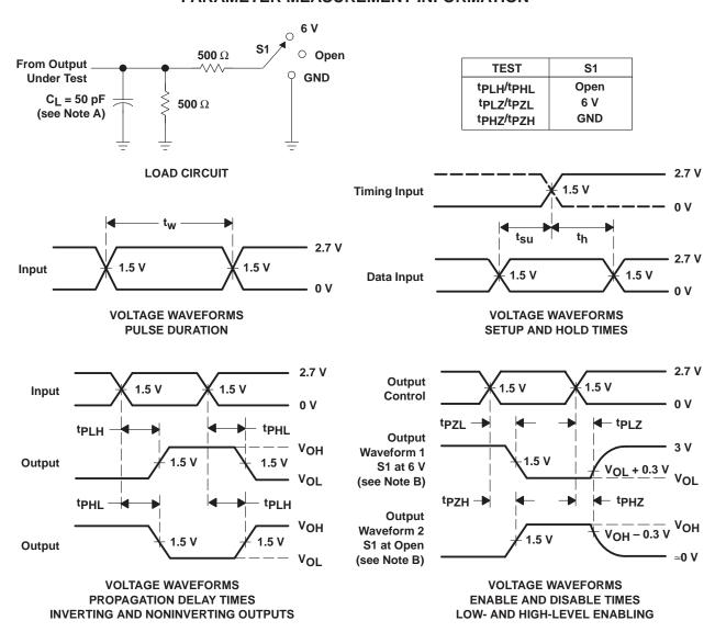
NOTES: B. C<sub>I</sub> includes probe and jig capacitance.
