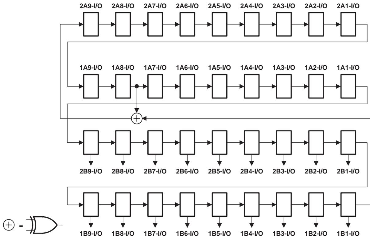
**Figure 5. 36-Bit PRPG Configuration ( $\overline{1OEAB} = \overline{2OEAB} = 0$ ,  $\overline{1OEB\overline{A}} = \overline{2OEB\overline{A}} = 1$ )**
