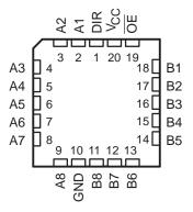
the B bus to the A bus, depending on the logic level at the direction-control (DIR) input. The output-enable  $(\overline{OE})$  input can be used to disable the devices so the buses are effectively isolated.
