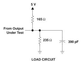
Figure 4. Equivalent AC Peak Output-Current Lumped Load
