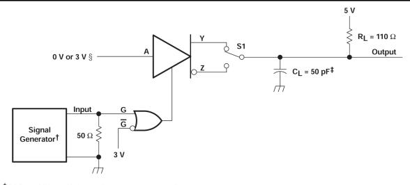
$<sup>^{\</sup>dagger}$  PRR = 1 MHz, 50% duty cycle,  $t_{\Gamma}$  < 6 ns,  $t_{f}$  < 6 ns,  $Z_{O}$  = 50  $\Omega$
