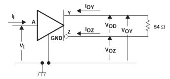
Figure 6-1. Test Circuit, V<sub>OD</sub> Without Common-Mode Loading
