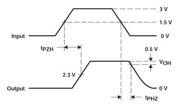
Figure 6-5. Enable Timing Test Circuit and Waveforms,  $t_{\mbox{\scriptsize PZH}}$  and  $t_{\mbox{\scriptsize PHZ}}$
