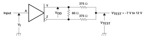
Figure 6-2. Test Circuit,  $V_{\text{OD}}$  With Common-Mode Loading
