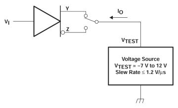
Figure 6-7. Test Circuit, Short-Circuit Output Current
