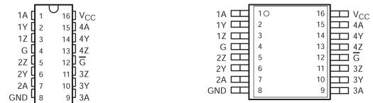
Figure 4-1. N Package (Top View)
