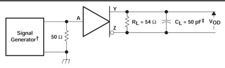
$<sup>^{\</sup>dagger}$  PRR = 1 MHz, 50% duty cycle,  $t_{r}$  < 6 ns,  $t_{f}$  < 6 ns,  $Z_{O}$  = 50  $\Omega$
