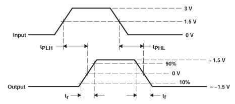
Figure 6-4. Output Switching Test Circuit and Waveforms
