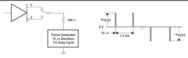
Figure 6-8. Test Circuit and Waveform, Transient Over-Voltage
