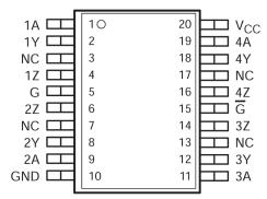
Figure 4-3. 20-DW Package (Top View)
