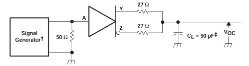
Figure 6-3. V<sub>OC</sub> Test Circuit
