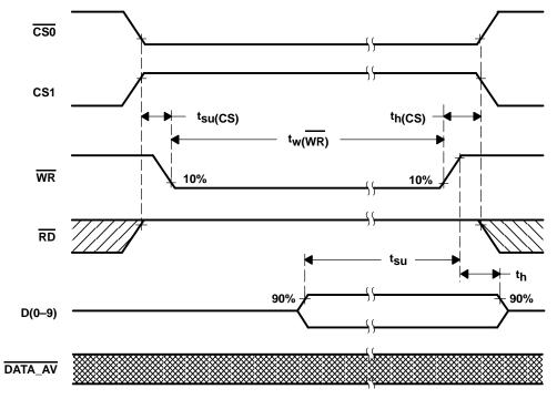
Figure 33. Write Timing Diagram Using WR (WR-controlled)
