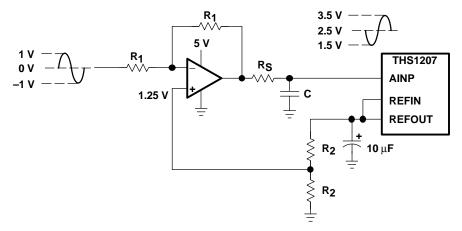
Figure 38. Level-Shift for DC-Coupled Input
