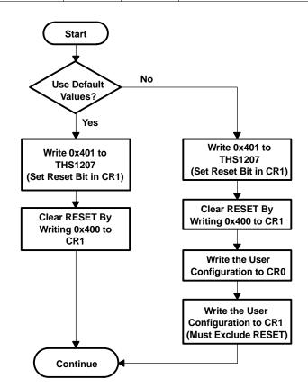
Figure 30. THS1207 Configuration Flow
