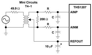
Figure 39. Transformer Coupled Input
