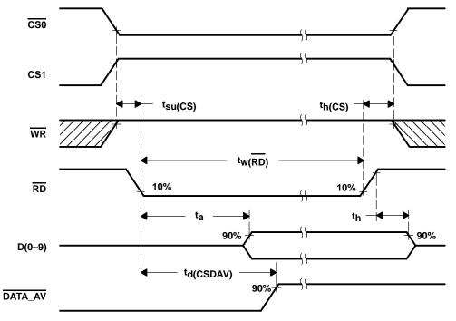
Figure 32. Read Timing Diagram Using RD (RD-controlled)
