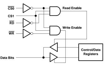
Figure 31. Logical Combination of  $\overline{CS0}$ , CS1,  $\overline{RD}$ , and  $\overline{WR}$
