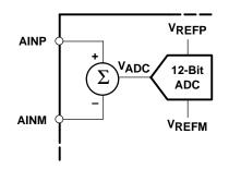
Figure 37. Differential Input Stage
