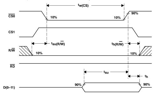
Figure 35. Write Timing Diagram Using R/W (CS0-controlled)
