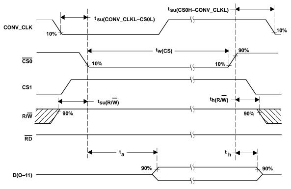
Figure 34. Read Timing Diagram Using R/W (CSO-controlled)
