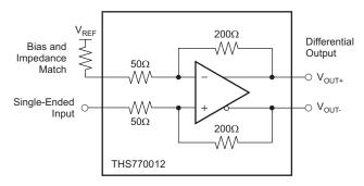
Figure 39. Single-Ended Input to Differential Output Amplifier
