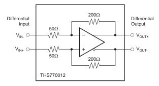
Figure 38. Differential Input to Differential Output Amplifier
