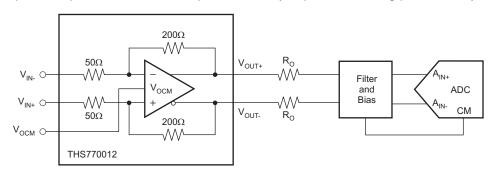
Figure 40. Generic ADC Driver Block Diagram
