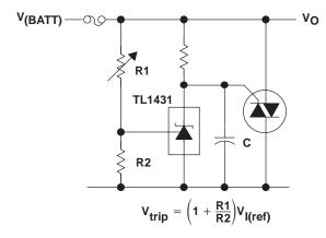
NOTE A: Refer to the stability boundary conditions in Figure 15 to determine allowable values for C.
