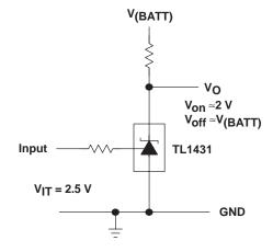
Figure 17. Single-Supply Comparator With Temperature-Compensated Threshold
