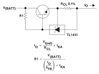
Figure 27. Precision Current Limiter
