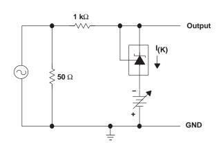
TEST CIRCUIT FOR REFERENCE IMPEDANCE
