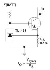
Figure 28. Precision Constant-Current Sink
