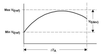
$\alpha_{V_{l(ref)}}$  is positive or negative, depending on whether minimum  $V_{l(ref)}$  or maximum  $V_{l(ref)}$ , respectively, occurs at the lower temperature.
