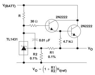
NOTE A: R should provide cathode current ≥1 mA to the TL1431 at minimum V(BATT).
