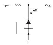
Figure 3. Test Circuit for Ioff
