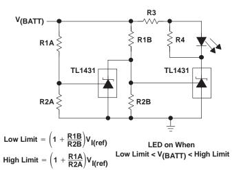
NOTE A: Select R3 and R4 to provide the desired LED intensity and cathode current ≥1 mA to the TL1431.
