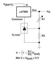
Figure 19. Output Control of a Three-Terminal Fixed Regulator
