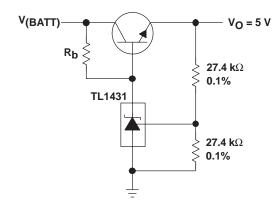
NOTE A:  $R_b$  should provide cathode current  $\geq$ 1 mA to the TL1431.
