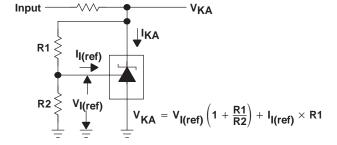
Figure 1. Test Circuit for  $V_{(KA)} = V_{ref}$
