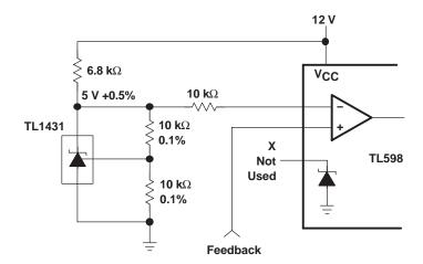
Figure 24. PWM Converter With 0.5% Reference
