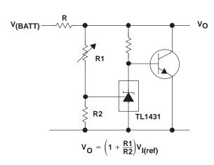
Figure 20. Higher-Current Shunt Regulator
