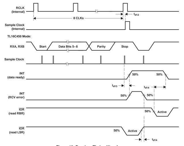
Figure 13. Receiver Timing Waveforms
