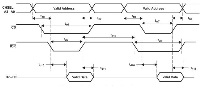
Figure 12. Read Cycle Timing Waveforms
