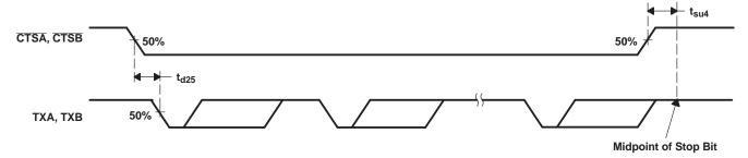
Figure 22. CTS and TX Autoflow Control Timing (Start and Stop) Waveforms
