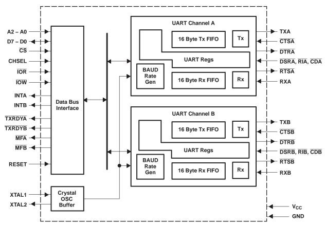
A. MF output allows selection of OP, BAUDOUT, or RXRDY per channel.
