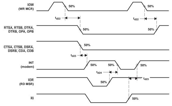
Figure 21. Modem Control Timing Waveforms
