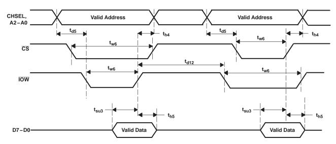
Figure 11. Write Cycle Timing Waveforms
