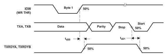
Figure 19. Transmitter Ready (TXRDY) Waveforms, FCR0 = 0 or FCR0 = 1 and FCR3 = 0 (Mode 0)
