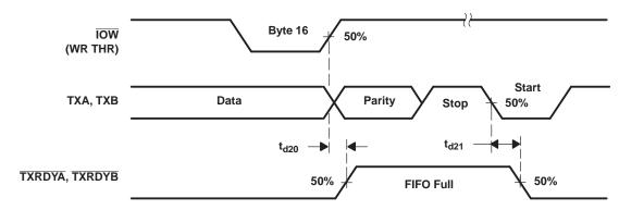
Figure 20. Transmitter Ready (TXRDY) Waveforms, FCR0 = 1 and FCR3 = 1 (Mode 1)
