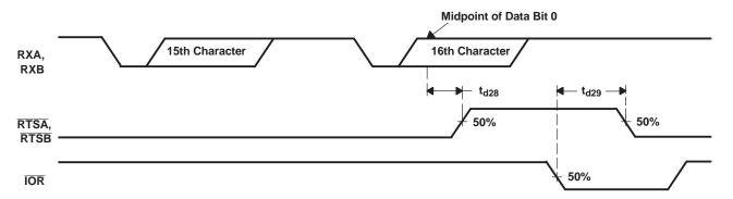
Figure 24. Auto-RTS Timing for RCV Threshold of 14 Waveforms
