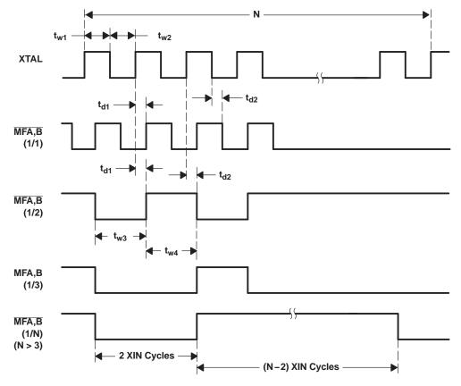
Figure 10. Input Clock and Baud Generator Timing Waveforms (For FN Package Only) (When AFR2:1 = 01)
