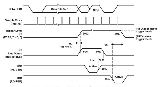
Figure 14. Receive FIFO First Byte (Sets DR Bit) Waveforms
