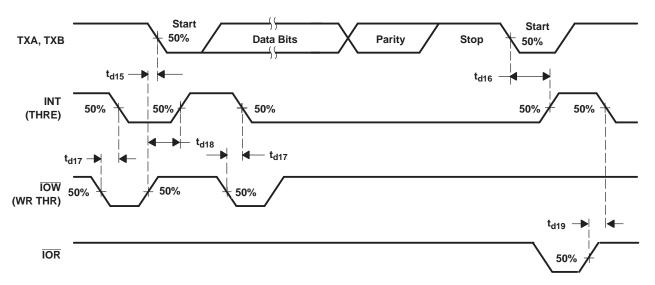
Figure 18. Transmitter Timing Waveforms
