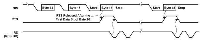
Figure 4. RTS Functional Timing Waveforms, RCV FIFO Trigger Level = 14 Bytes
