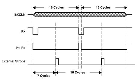
Figure 32. Recommended Strobing For Decoded Data
