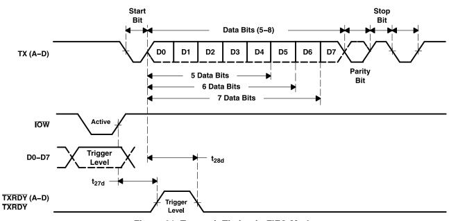
Figure 21. Transmit Timing in FIFO Mode
