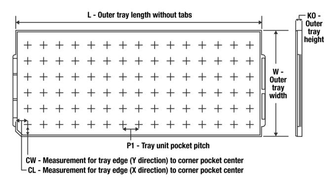
Chamfer on Tray corner indicates Pin 1 orientation of packed units.
