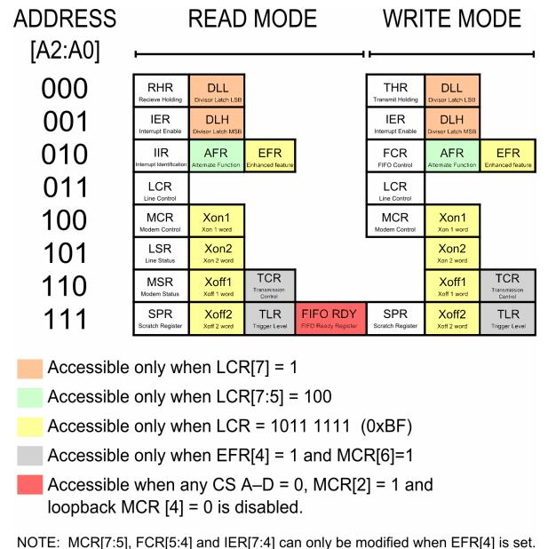
Figure 22. Register Map – Read and Write Properties
