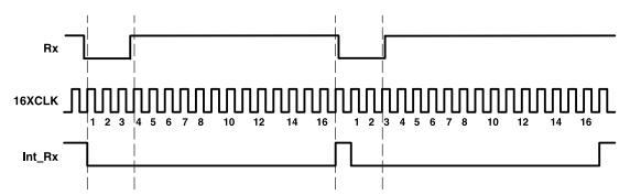
Figure 31. Timing Causing 1-Clock-Wide Pulse Between Consecutive Ones
