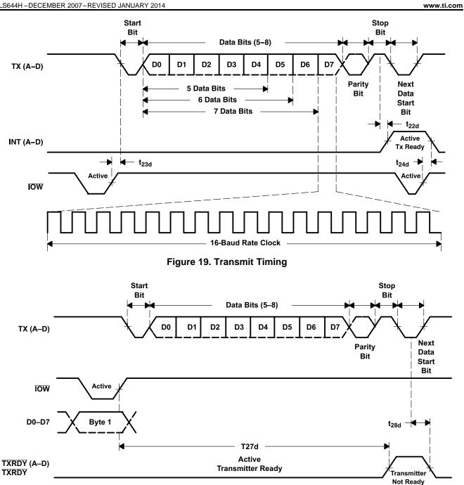
Figure 20. Transmit Ready Timing in None FIFO Mode
