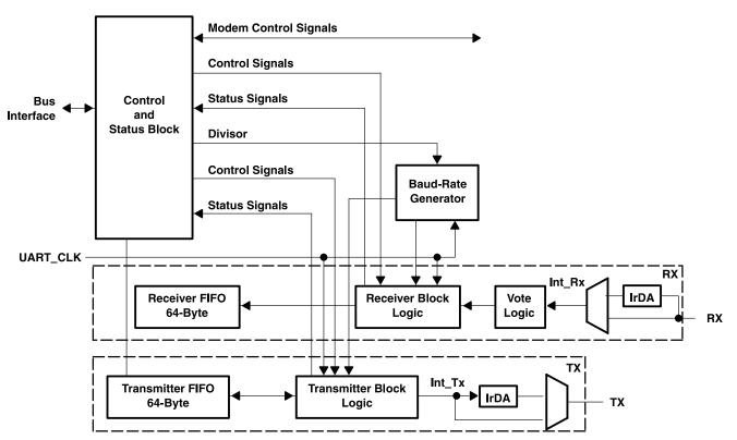
A. The vote logic determines whether the RX data is a logic 1 or 0. It takes three samples of the RX line and uses a majority vote to determine the logic level received. The vote logic operates on all bits received.
