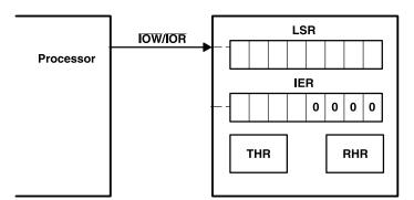
Figure 6. FIFO Polled Mode Operation
