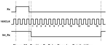
Figure 33. Positive Rx Pulse Decode – Detailed View
