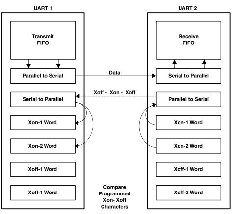
Figure 4. Software Flow Control Example
