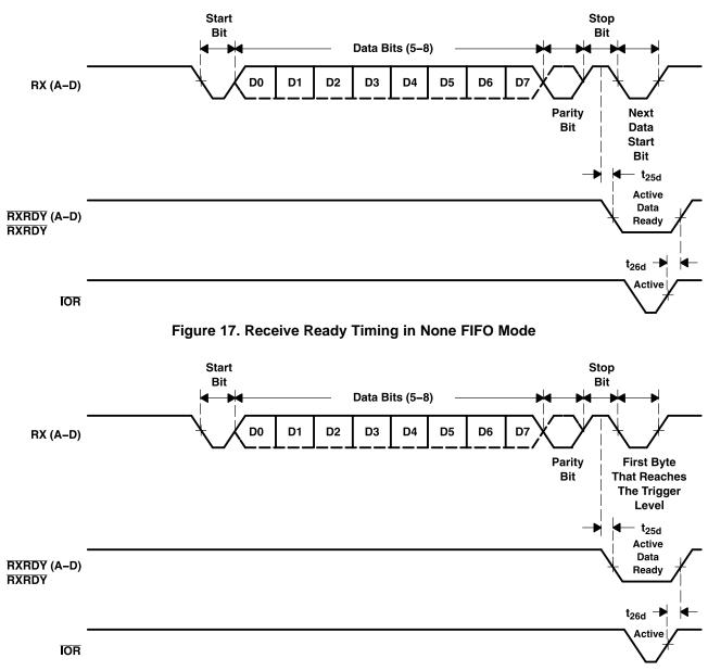
Figure 18. Receive Timing in FIFO Mode
