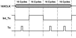
Figure 27. IrDA-SIR Encoding Scheme – Detailed Timing Diagram
