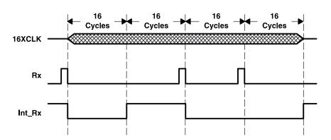
Figure 34. Positive Rx Pulse Decode – Macro View
