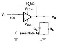
NOTE A: C<sub>L</sub> includes fixture capacitance.
