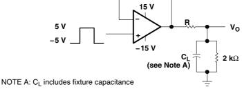
Figure 44. Test Circuit for Output Characteristics
