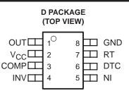
The TL5002 incorporates on a single monolithic chip all the functions required for a pulse-width-modulation (PWM) control circuit. Designed primarily for power-supply control, the TL5002 contains an error amplifier, a regulator, an oscillator, a PWM comparator with a dead-time-control input, undervoltage lockout (UVLO), and an open-collector output transistor.
