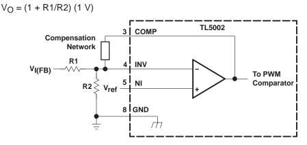
Figure 1. Error-Amplifier Gain Setting
