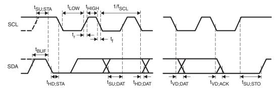
Rise and fall times refer to  $V_{\text{IL}}$  and  $V_{\text{IH}}$ .
