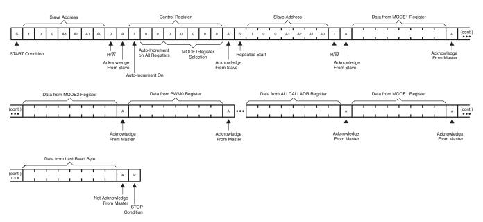
Figure 17. Read All Registers With the Auto-Increment Feature
