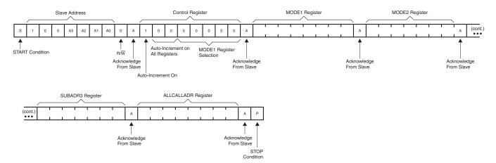
Figure 15. Write to All Registers Using Auto-Increment
