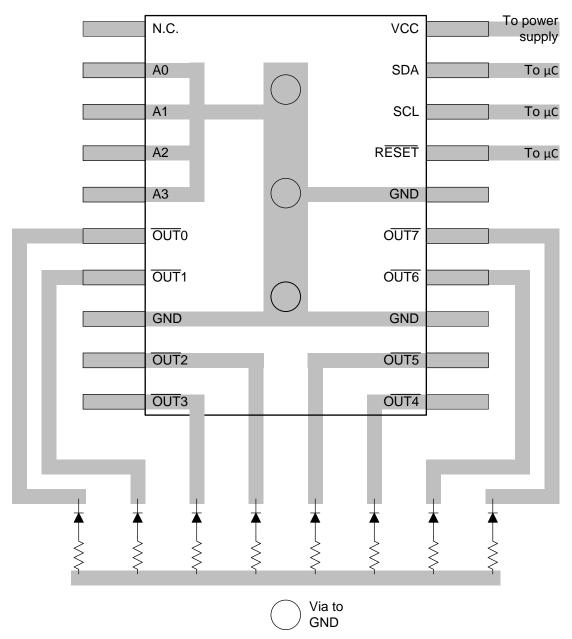
Figure 26. PW Layout Example
