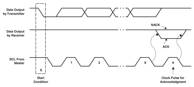
Figure 13. Acknowledge on I<sup>2</sup>C Bus
