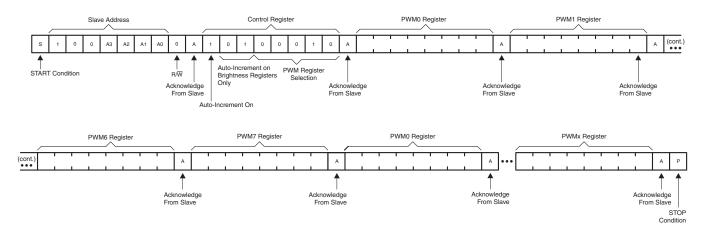
Figure 16. Multiple Writes to Individual Brightness Registers Only Using the Auto-Increment Feature
