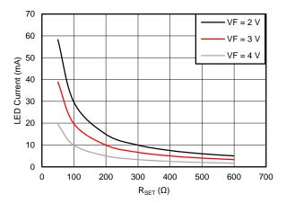
Figure 24. LED Current vs R<sub>SET</sub>
