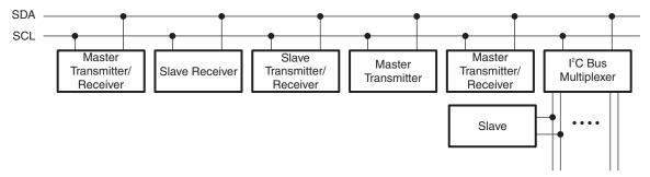
Figure 12. System Configuration
