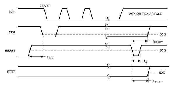
Figure 3. Definition of Reset Timing
