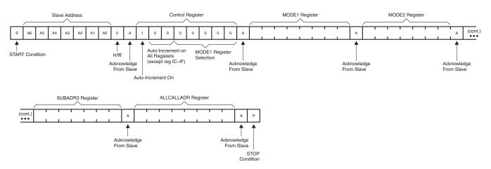
Figure 13. Write to All Registers Using Auto-Increment
