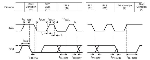
NOTE: Rise and fall times refer to  $V_{\text{IL}}$  and  $V_{\text{IH}}$ .
