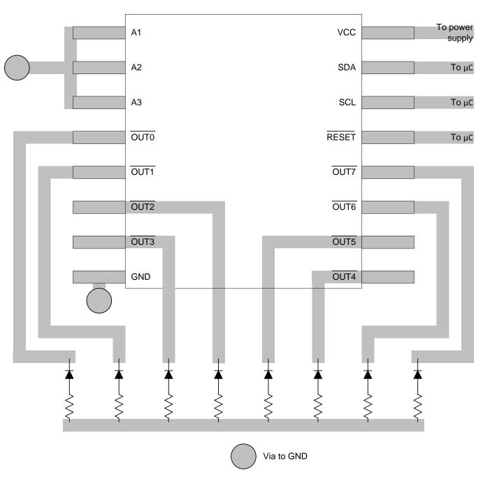
Figure 23. PW Layout Example
