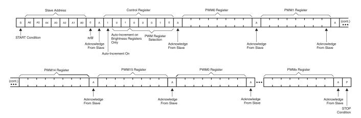
Figure 14. Multiple Writes to Individual Brightness Registers Only Using the Auto-Increment Feature
