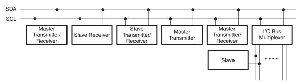
Figure 10. System Configuration
