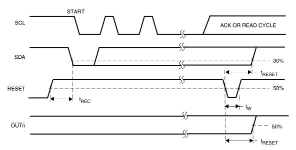
Figure 1. Definition of RESET Timing
