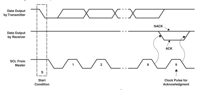
Figure 11. Acknowledge on I<sup>2</sup>C Bus
