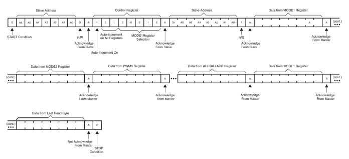
Figure 15. Read All Registers With the Auto-Increment Feature
