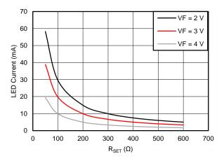
Figure 21. LED Current vs R<sub>SET</sub>
