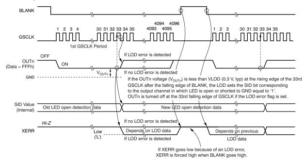
Figure 31. LED Open Detection (LOD) Timing
