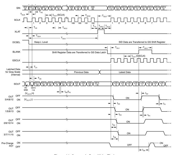
Figure 14. Grayscale Data Write Timing
