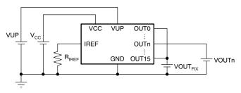
Figure 10. Leakage Current of Pre-Charge FET Test Circuit for OUTn
