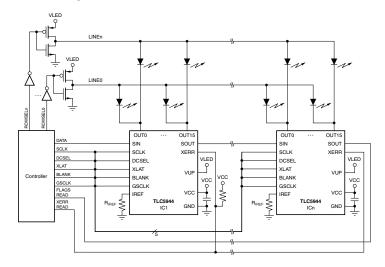
Typical Application Circuit (Multiple Daisy-Chained TLC5944s)
