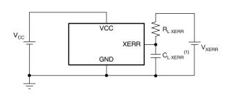
(1)  $C_{L\ XERR}$  includes measurement probe and jig capacitance. Figure 7. Fall Time Test Circuit for XERR
