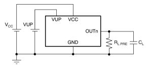
Figure 8. Delay Time Test Circuit for Pre-Charge FET
