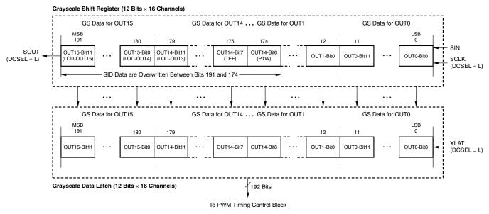
Figure 28. Grayscale Shift Register and Data Latch Configuration
