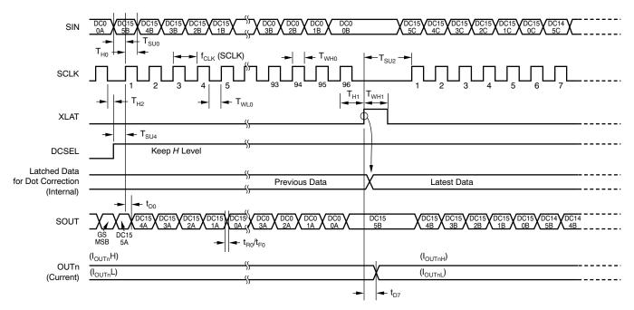
Figure 15. Dot Correction Data Write Timing
