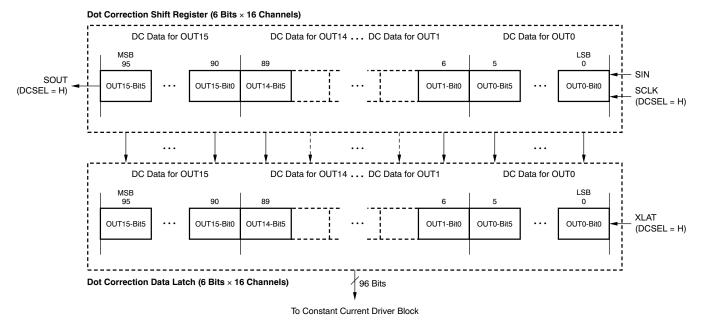
Figure 29. Dot Correction Shift Register and Latch Configuration
