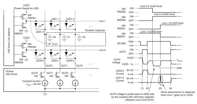
Figure 33. LED Ghost-Lighting Phenomenon Mechanism
