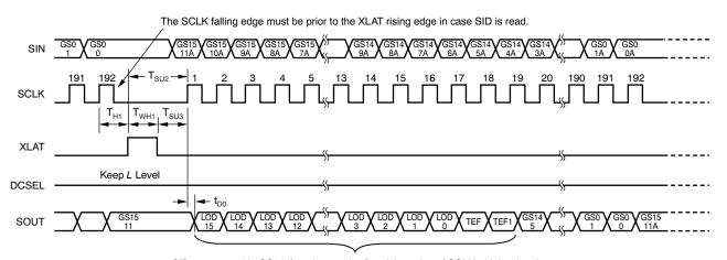
SID are entered in GS shift register at the first rising edge of SCLK with low level of DCSEL after XLAT. The SID readout consists of the saved LOD result at the 33rd GSCLK rising edge in the previous display period and the saved TEF data and TEF1 at the rising edge of the first of SCLK after XLAT goes low.
