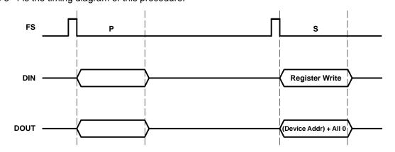
Figure 3–4. Device 3/Register 1 Write Operation Timing Diagram
