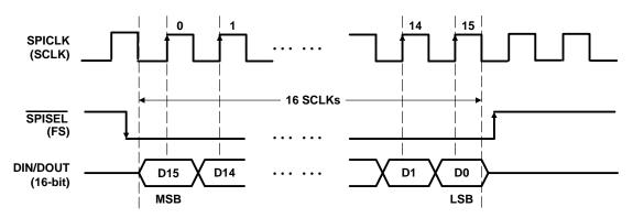
Figure 2–11. Timing Diagram for the SPI\_CP1 Mode (M1M0 = 10)
