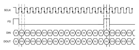
Figure 3–10. Continuous Data Transfer Mode Timing
