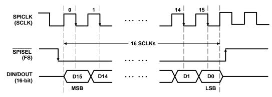
Figure 2–10. Timing Diagram for the SPI\_CP0 Mode (M1M0 = 01)
