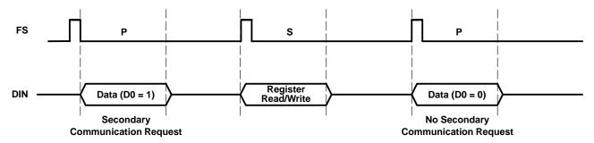
Figure 3–7. FS Output During Software Secondary Serial Communication Request (No Slave)
