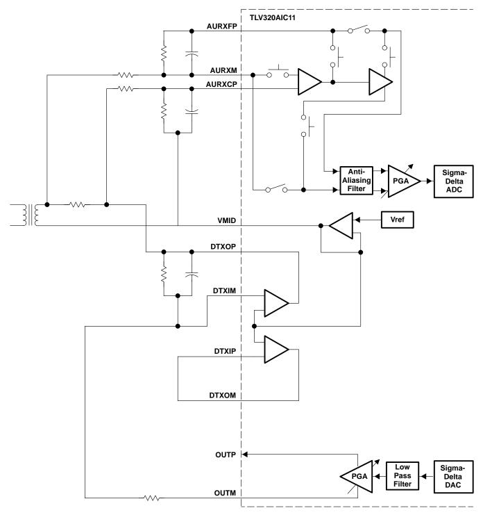
Figure A–2. Single-Ended Configuration of Hybrid Connection
