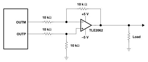
Figure 2–18. Differential Output Drive (Ground-Referenced)
