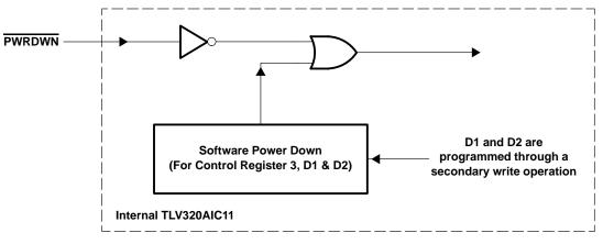
Figure 2–8. Internal Power-Down Logic
