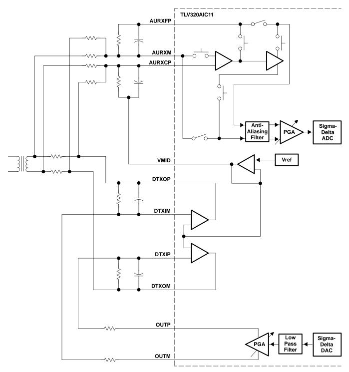
Figure A–1. Differential Configuration for Hybrid Connection
