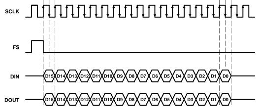
Figure 3–1. Primary Serial Communication Timing
