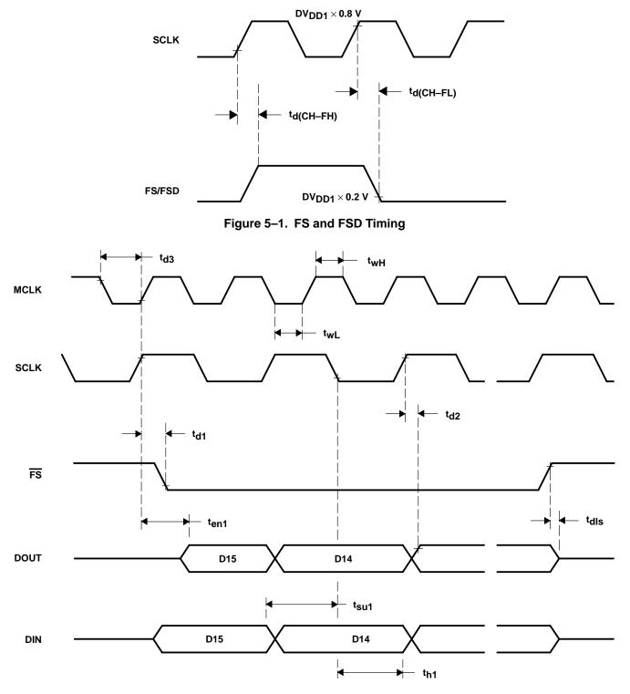
Figure 5–2. Serial Communication Timing
