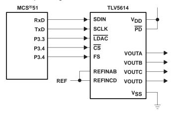
Figure 19. TLV5614 Interfaced With MCS®51
