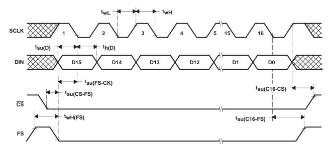
Figure 2. Timing Diagram
