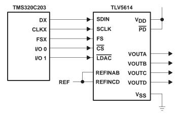
Figure 18. TLV5614 Interfaced With TMS320C203
