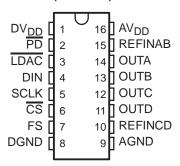
reference buffers, and output buffers (via pins  $AV_{DD}$  and AGND). Each supply is independent of the other and can be any value between 2.7 V and 5.5 V. The dual supplies allow a typical application where the DAC is controlled via a microprocessor operating on a 3-V supply (also used on pins DV<sub>DD</sub> and DGND), with the DACs operating on a 5-V supply. The digital and analog supplies can be tied together.
