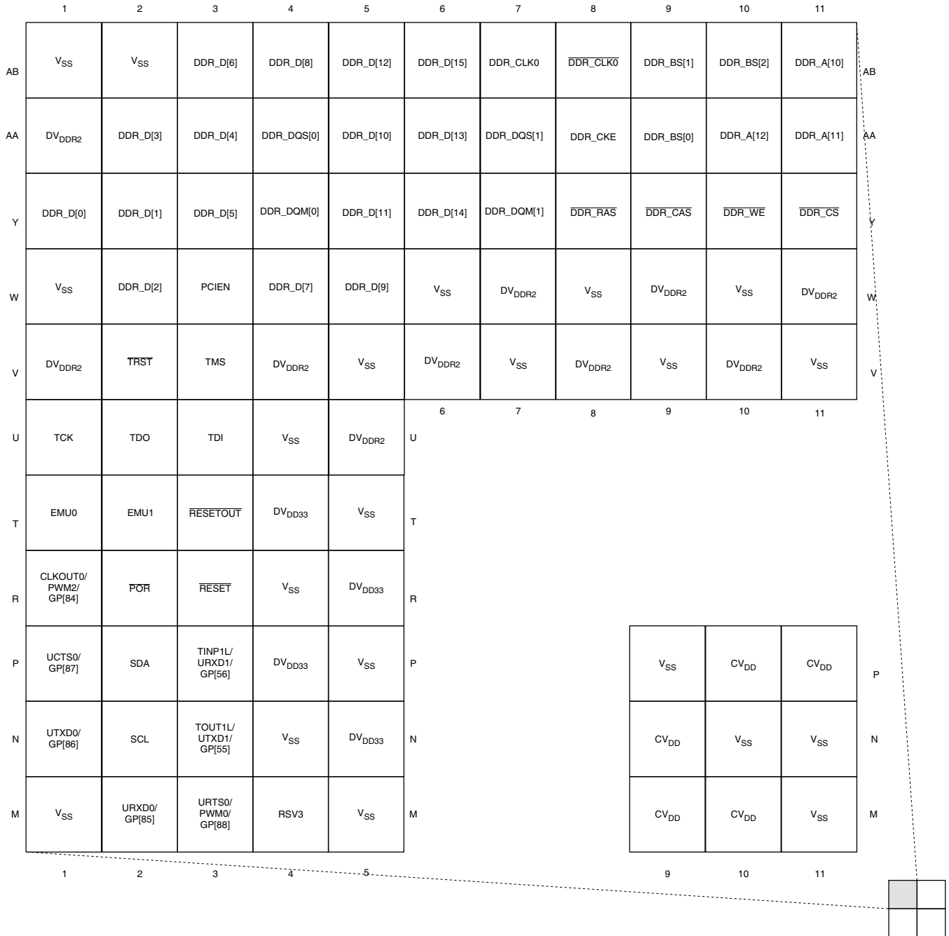
Figure 2-10. ZDU Pin Map [Quadrant A]
