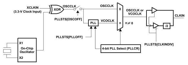
Figure 6-17. OSC and PLL Block Diagram
