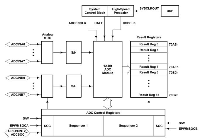
Figure 6-5. Block Diagram of the ADC Module
