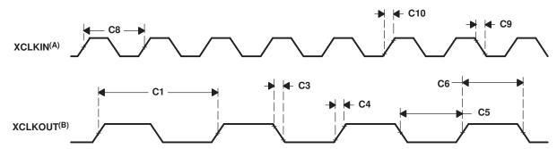
A. The relationship of XCLKIN to XCLKOUT depends on the divide factor chosen. The waveform relationship shown is intended to illustrate the timing parameters only and may differ based on actual configuration.
