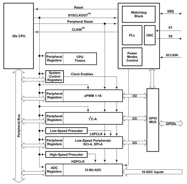
A. CLKIN is the clock into the CPU. It is passed out of the CPU as SYSCLKOUT (that is, CLKIN is the same frequency as SYSCLKOUT).
