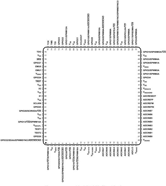
Figure 4-1. 100-Pin PZ LQFP (Top View)
