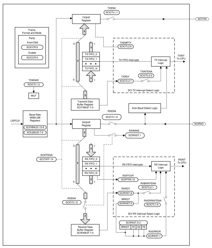
Figure 6-8. Serial Communications Interface (SCI) Module Block Diagram
