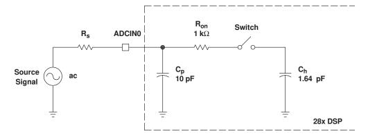
Typical Values of the Input Circuit Components:
