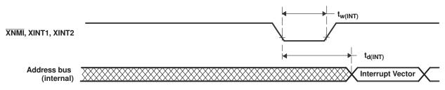
Figure 5-14. External Interrupt Timing
