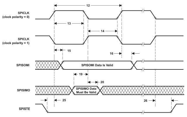
Figure 5-17. SPI Slave Mode External Timing (Clock Phase = 0)
