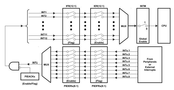
Figure 6-15. Multiplexing of Interrupts Using the PIE Block
