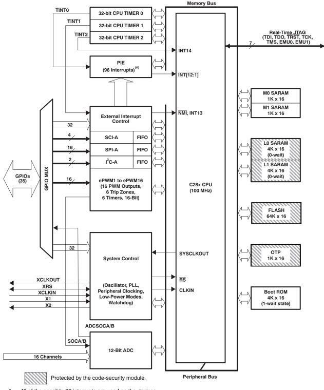
A. 43 of the possible 96 interrupts are used on the devices.
