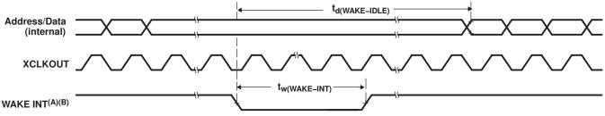
A. WAKE INT can be any enabled interrupt, WDINT, XNMI, or XRS.
