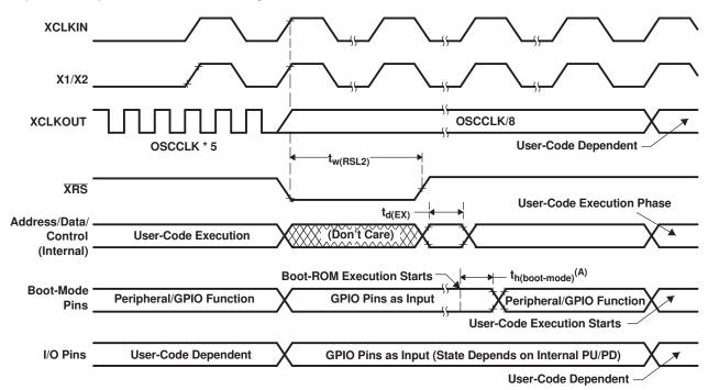
After reset, the Boot ROM code samples BOOT Mode pins. Based on the status of the Boot Mode pin, the boot code Α. branches to destination memory or boot code function. If Boot ROM code executes after power-on conditions (in debugger environment), the Boot code execution time is based on the current SYSCLKOUT speed. The SYSCLKOUT will be based on user environment and could be with or without PLL enabled.
