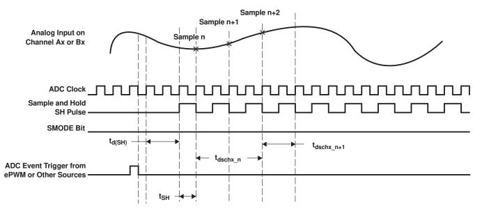
Figure 5-22. Sequential Sampling Mode (Single-Channel) Timing
