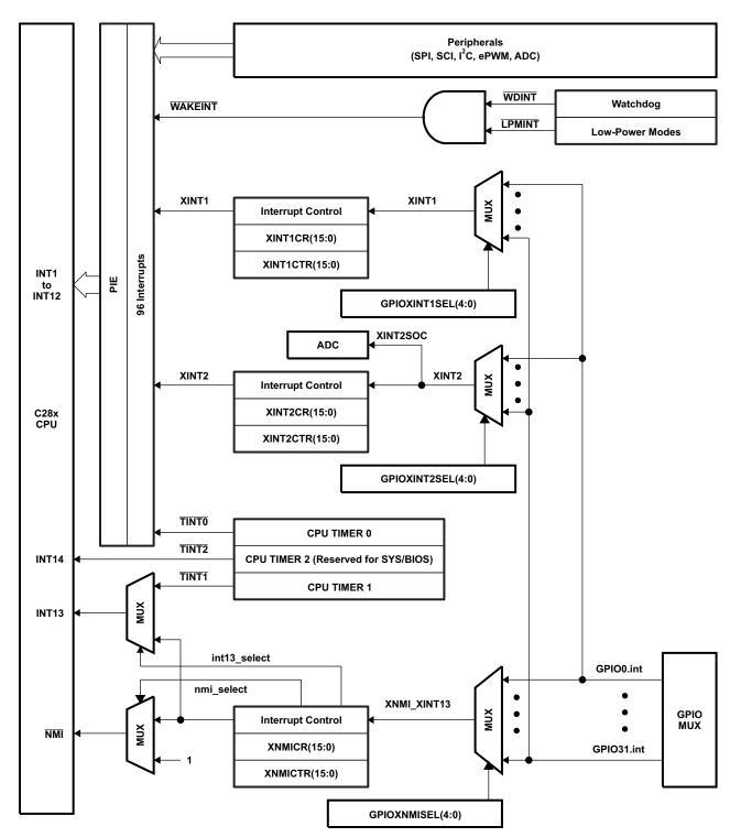
Figure 6-14. External and PIE Interrupt Sources
