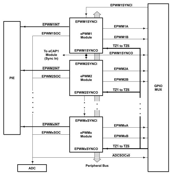
Figure 6-3. Multiple PWM Modules
