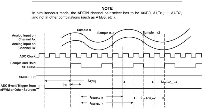
Figure 5-23. Simultaneous Sampling Mode Timing
