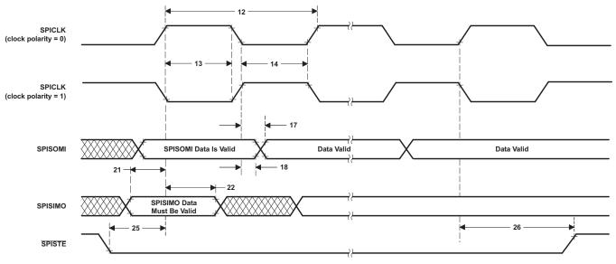
Figure 5-18. SPI Slave Mode External Timing (Clock Phase = 1)
