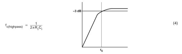
The value of C<sub>i</sub> is important to consider as it directly affects the bass (low frequency) performance of the circuit. Consider the example where R<sub>i</sub> is 10 k $\Omega$  and the specification calls for a flat bass response down to 40 Hz. Equation 2 is reconfigured as equation 5.
