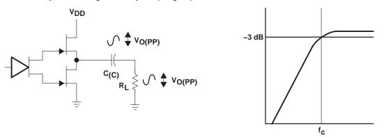
Figure 25. Single-Ended Configuration and Frequency Response
