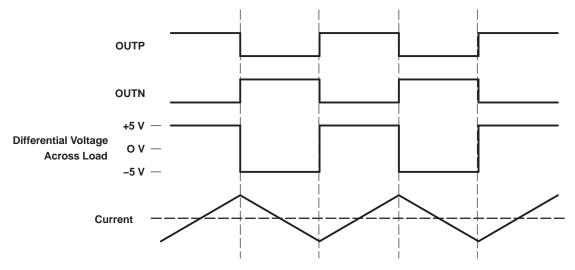
Figure 9. Traditional Class-D Modulation Scheme's Output Voltage and Current Waveforms Into an Inductive Load With No Input
