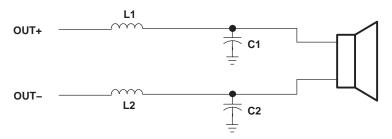
Figure 11. Class-D Output Filter
