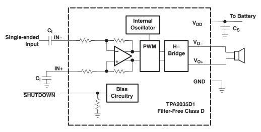
Figure 31. TPA2035D1 Application Schematic With Single-Ended Input
