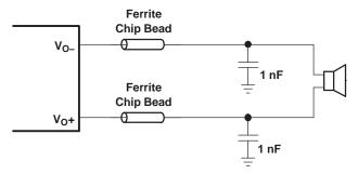
Figure 34. Typical Ferrite Chip Bead Filter
