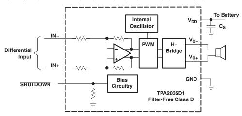
Figure 29. Typical TPA2035D1 Application Schematic With Differential Input for a Wireless Phone
