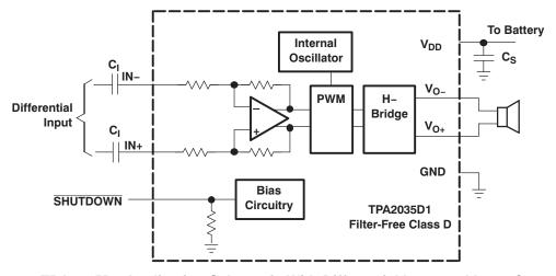
Figure 30. TPA2035D1 Application Schematic With Differential Input and Input Capacitors
