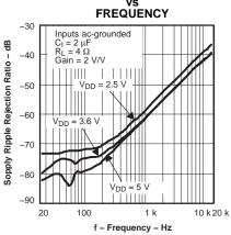
SUPPLY RIPPLE REJECTION RATIO vs FREQUENCY
