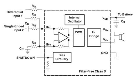
Figure 31. Application Schematic With TPA2036D1 Summing Differential Input and Single-Ended Input Signals
