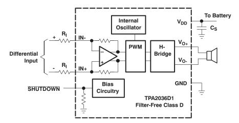
Figure 27. Typical TPA2036D1 Application Schematic With Differential Input for a Wireless Phone
