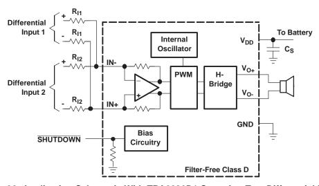
Figure 30. Application Schematic With TPA2036D1 Summing Two Differential Inputs
