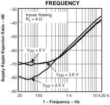
**GSM POWER SUPPLY REJECTION**
