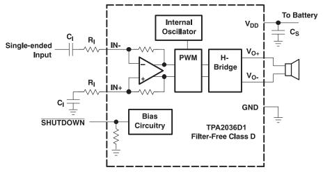
Figure 29. TPA2036D1 Application Schematic With Single-Ended Input
