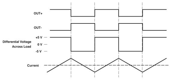
Figure 35. Traditional Class-D Modulation Scheme's Output Voltage and Current Waveforms Into an Inductive Load With no Input
