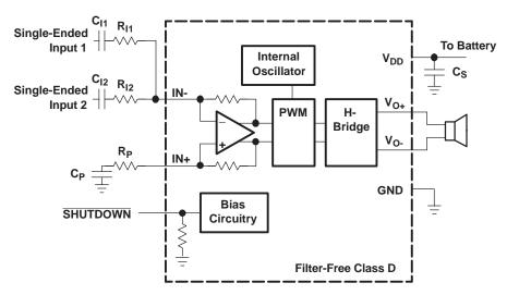
Figure 32. Application Schematic With TPA2036D1 Summing Two Single-Ended Inputs
