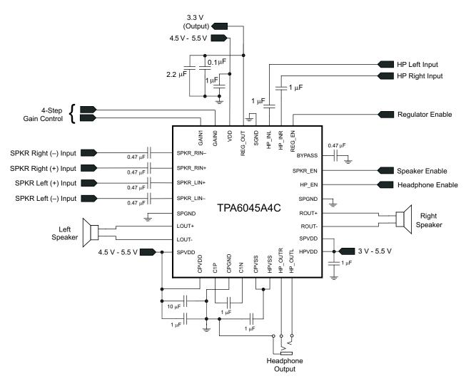
Figure 39. Differential Input Application Circuit
