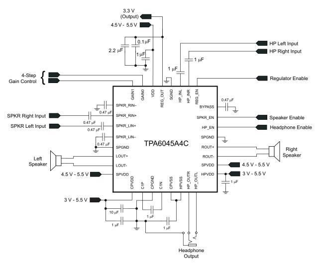
Figure 38. Single-Ended Input Application Circuit
