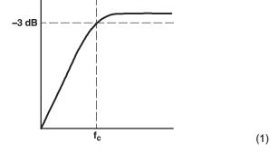
The value of  $C_1$  is important to consider as it directly affects the low-frequency, or bass, performance of the circuit. Furthermore, the input impedance changes with a change in volume. The higher the volume, the lower the input impedance is. To determine the appropriate capacitor value, reconfigure Equation 1 into Equation 2. The value of the input resistor,  $R_1$ , can be determined from Equation 2.
