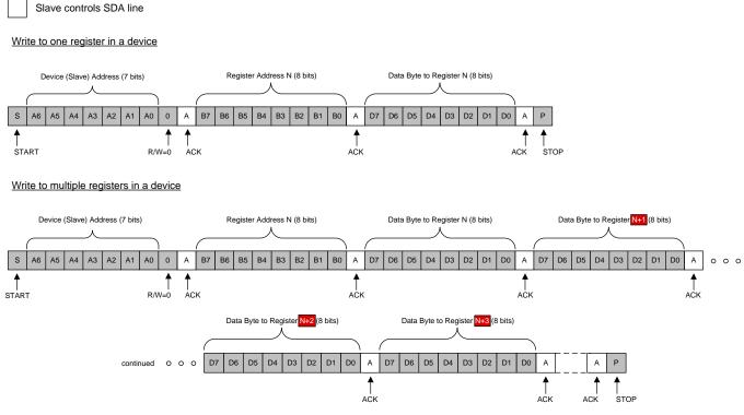
Figure 26. Write Operation to One or Multiple Registers
