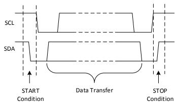
Figure 22. Definition of START and STOP Conditions
