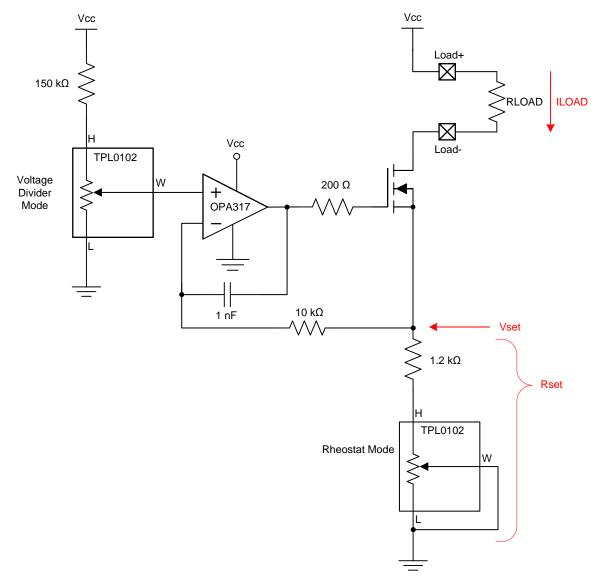
Figure 35. Variable Current Sink Schematic
