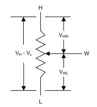
Figure 19. Equivalent Circuit for Voltage Divider Mode
