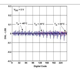
Figure 2. Voltage Divider Mode DNL vs Digital Code ( $V_{DD}$  = 5
