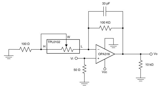
Figure 31. Gain Control Compensation Schematic
