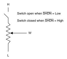
Figure 18. Equivalent Circuit for Shutdown Mode
