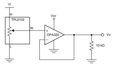
Figure 33. Digital to Analog Converter Schematic
