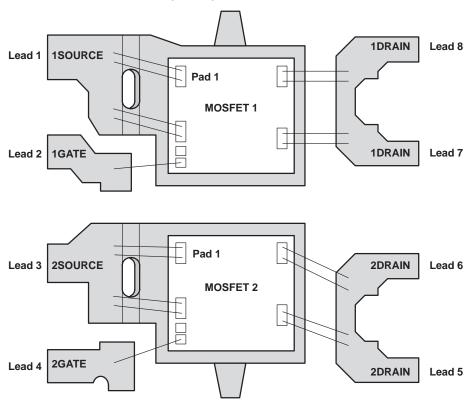
Figure 16. TPS1120 Dual MOSFET SO-8 Lead Frame
