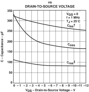
$\dagger C_{iss} = C_{gs} + C_{gd}, C_{ds(shorted)}$  $\ddagger C_{rss} = C_{gd}, C_{oss} = C_{ds} + \frac{C_{gs} C_{gd}}{C_{gs} + C_{gd}} \approx C_{ds} + C_{gd}$ Figure 6
