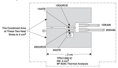
Figure 14. Profile of Heat Sinks
