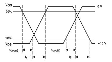
Figure 2. Switching-Time Waveforms
