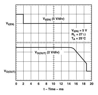
Figure 3. Turnoff Delay and Fall Time
