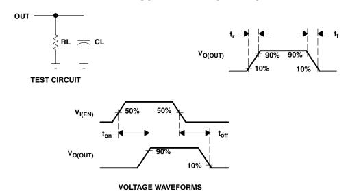
Figure 1. Test Circuit and Voltage Waveforms
