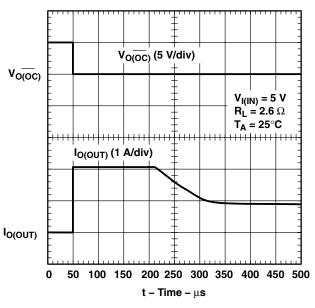
Figure 16. 2.6-Ω Load Connected to an Enabled TPS2031 Device
