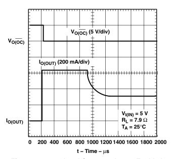
Figure 13. 7.9-Ω Load Connected to an Enabled TPS2030 Device
