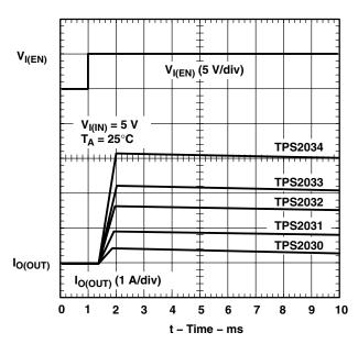
Figure 6. Device Enabled Into Short
