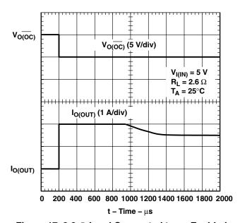
Figure 17. 2.6-Ω Load Connected to an Enabled TPS2032 Device
