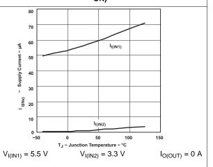
Figure 12. Supply Current vs Junction Temperature (Device Disabled)
