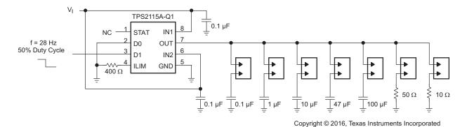
Figure 17. Output Switchover Voltage Droop vs Load Capacitance Test Circuit
