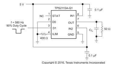
Figure 16. Output Switchover Voltage Droop Test Circuit
