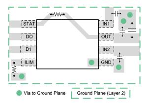
Figure 24. TPS2115A-Q1 Layout Example
