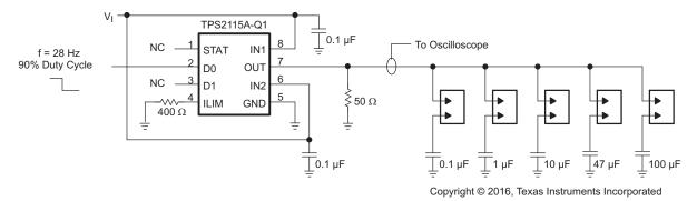
Figure 19. Output Capacitance Inrush Current vs Load Capacitance Test Circuit
