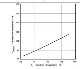
Figure 8. Switch On-Resistance vs Junction Temperature
