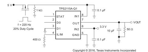
Figure 18. Auto Switchover Voltage Drop Test Circuit
