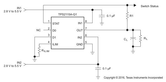
Figure 20. Auto-Selecting for a Dual Power Supply Application
