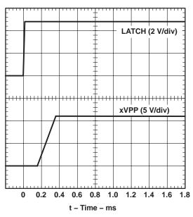
Figure 15. xVPP Propagation Delay and Rise Time With 1-µF Load, 12-V Switch
