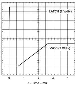
Figure 11. xVCC Propagation Delay and Rise Time With 1-µF Load, 5-V Switch
