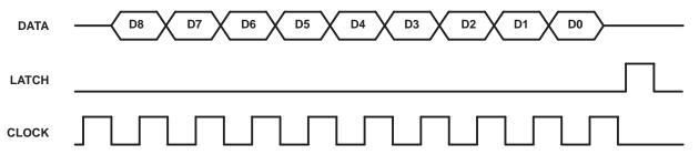
NOTE A: Data is clocked in on the positive leading edge of the clock. The latch should occur before the next positive leading edge of the clock. For definition of D0 to D8, see the control logic table.
