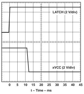
Figure 12. xVCC Propagation Delay and Fall Time With 1-µF Load, 5-V Switch
