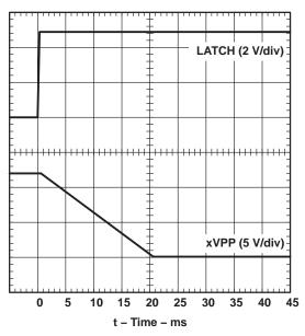
Figure 18. xVPP Propagation Delay and Fall Time With 150-µF Load, 12-V Switch
