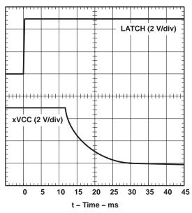
Figure 14. xVCC Propagation Delay and Fall Time With 150-µF Load, 5-V Switch
