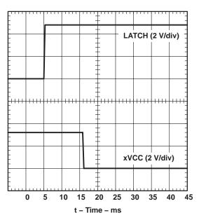
Figure 4. xVCC Propagation Delay and Fall Time With 1-µF Load, 3.3-V Switch,  $(V_{I(5V)} = 5 V)$
