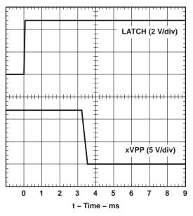
Figure 16. xVPP Propagation Delay and Fall Time With 1-µF Load, 12-V Switch
