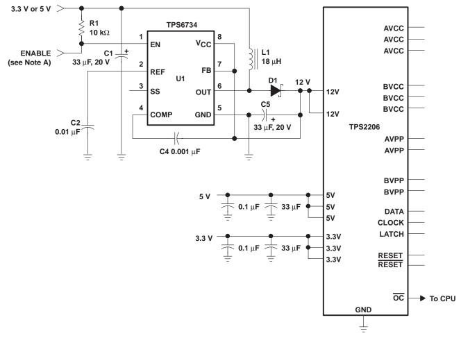
NOTE A: The enable terminal can be tied to a generall purpose I/O terminal on the PCMCIA controller or tied high.
