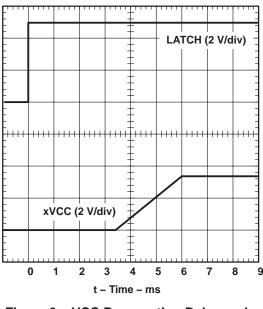
Figure 3. xVCC Propagation Delay and Rise Time With 1- $\mu\text{F}$  Load, 3.3-V Switch,  $(V_{I(5V)} = 5 V)$
