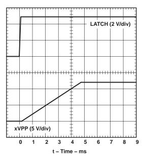
Figure 17. xVPP Propagation Delay and Rise Time With 150-µF Load, 12-V Switch
