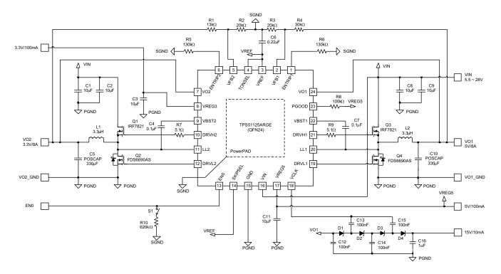
Figure 42. 5-V/8-A, 3.3-V/8-A Application Circuit (245-kHz/305-kHz Setting)
