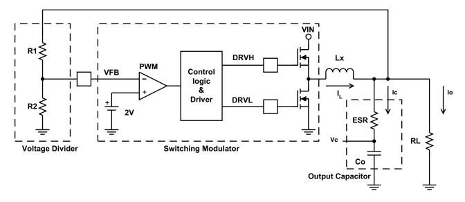
Figure 37. Simplifying the Modulator
