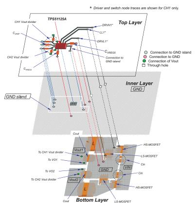
Figure 41. PCB Layout Design
