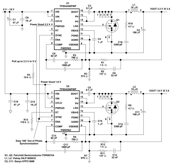
Figure 26. 3.3-V/1.8-V Power Supply With Sequencing
