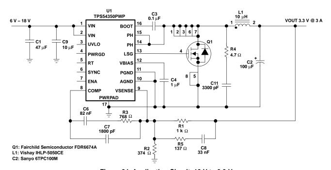
Figure 24. Application Circuit, 12 V to 3.3 V
