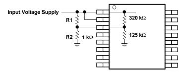
Figure 1. Circuit Using External UVLO Function
