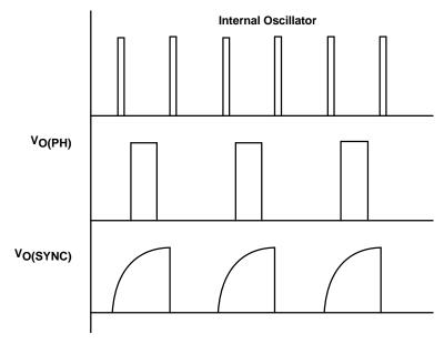
Figure 4. SYNC Output Waveform
