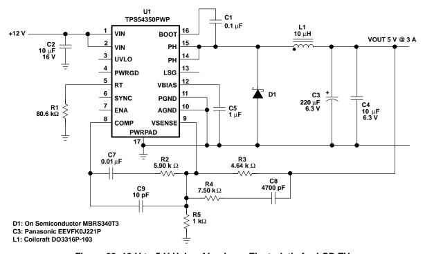
Figure 28. 12-V to 5-V Using Aluminum Electrolytic for LCD TV
