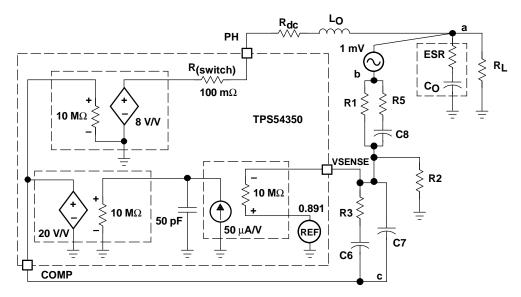
Figure 23. Model of Control Loop
