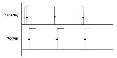
Figure 3. SYNC Input Waveform
