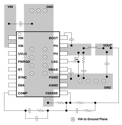
Figure 21. TPS54350 PCB Layout
