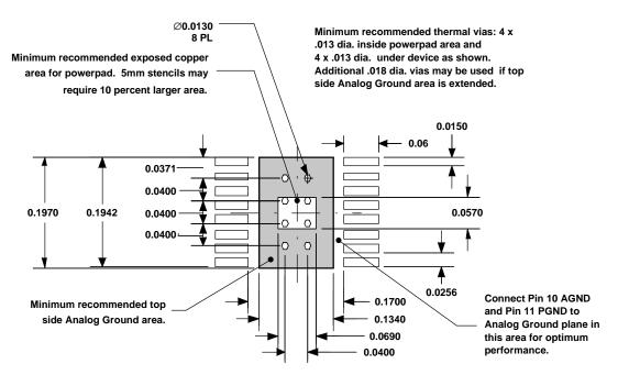
Figure 22. Thermal Considerations for PowerPAD Layout
