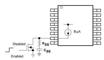
Figure 2. Interfacing to the ENA Pin
