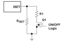
Figure 13. Switching In/Out an Additional Resistor to Change Output Current
