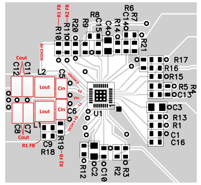
Figure 34. Layout Example From EVM for TPS6505x
