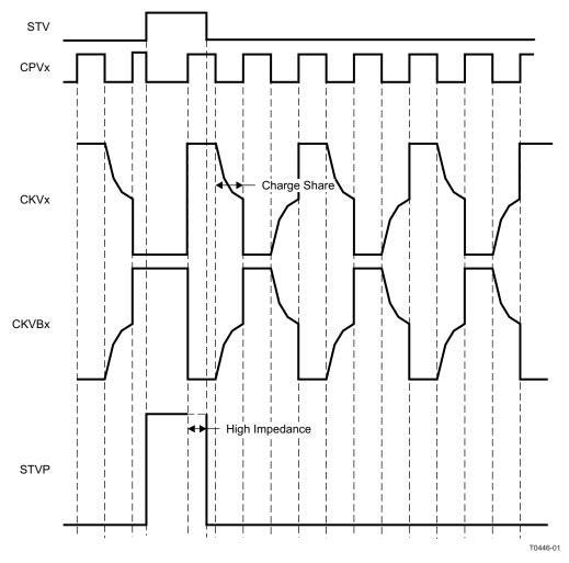
Figure 21. Scan Driver Timing Diagram
