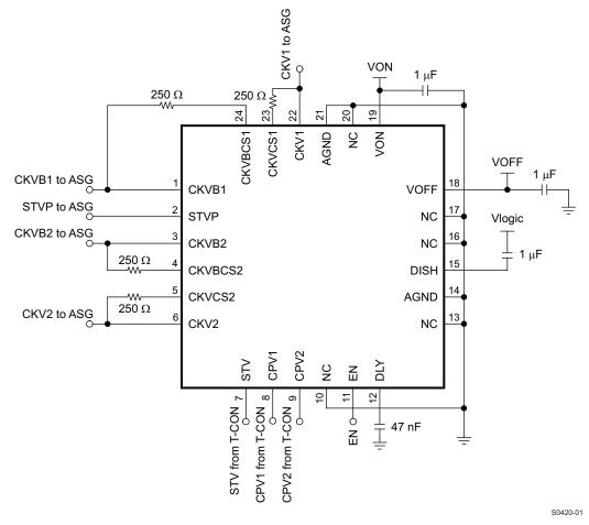
Figure 24. Typical Application With VOFF Discharge Enabled
