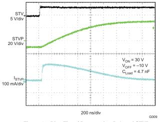
Figure 12. Rise Time / Propagation Delay of STVP, CPV1 = LOW
