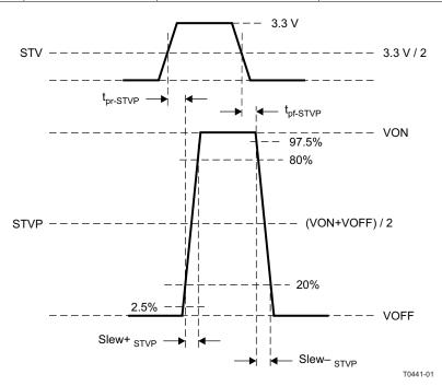
Figure 1. Switching Characteristics of STVP
