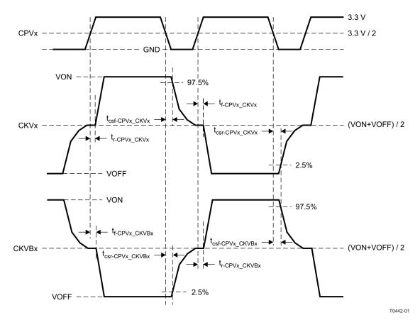
Figure 2. Switching Characteristics of CKVx, CKVBx (STV = GND)
