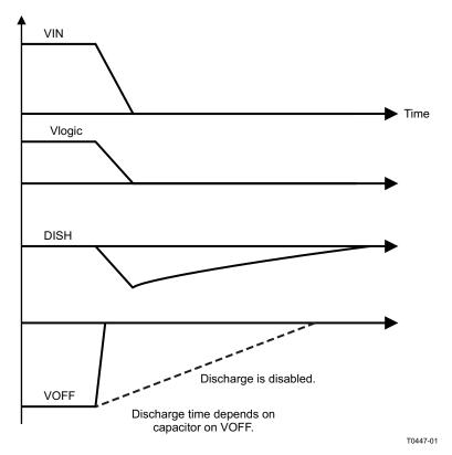
Figure 23. Power-Off Sequence of VOFF Discharge
