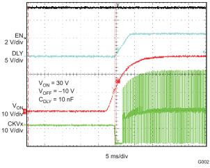
Figure 5. Start-Up Sequence CKVx, EN = HIGH Before UVLO
