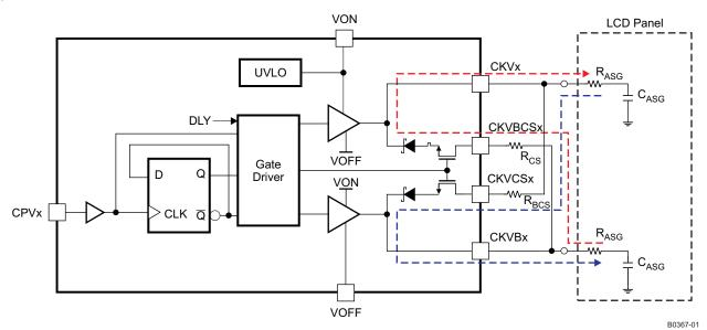
Figure 18. Single-Scan Driver Block Diagram
