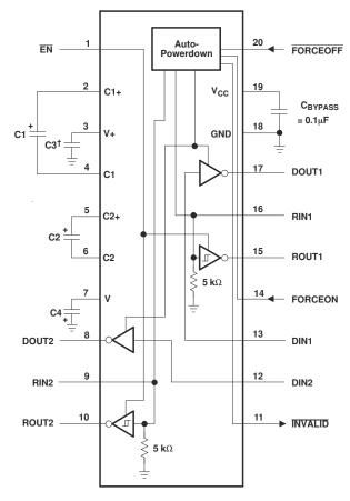
$<sup>^{\</sup>dagger}$  C3 can be connected to  $V_{CC}$  or GND.
