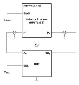
Figure 8. Test Circuit for Frequency Response (BW)
