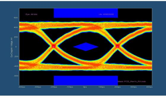
Figure 4. Transitional Signal Eye for TS2PCIE412 Using a 10-inch Trace
