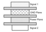
Figure 12. Four-Layer Board Stackup
