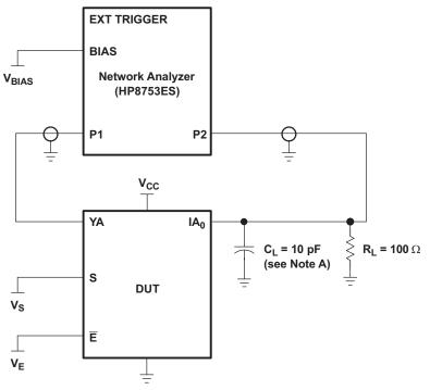
A. C<sub>L</sub> includes probe and jig capacitance.
