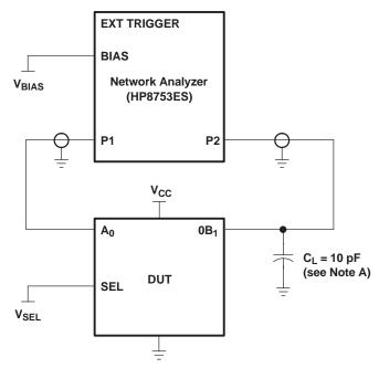
A.  $C_L$  includes probe and jig capacitance.
