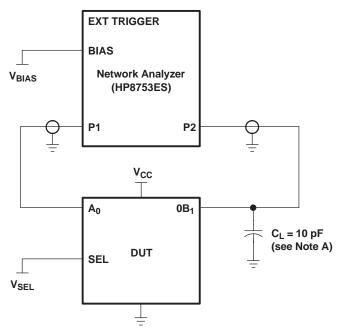
A. C<sub>L</sub> includes probe and jig capacitance.
