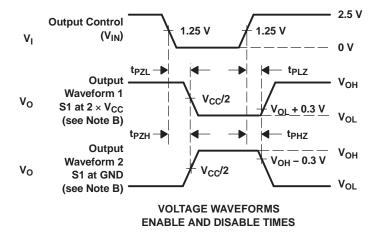
NOTES: A. C<sub>I</sub> includes probe and jig capacitance.
