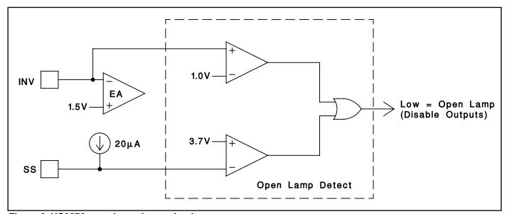
Figure 3. UC3872 open lamp detect circuitry.
