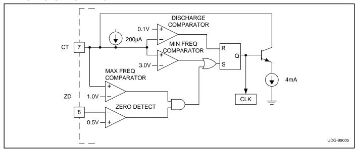
Figure 2. UC3872 oscillator section.
