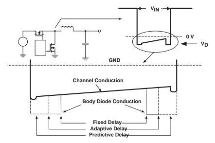
Figure 7. Switch Node Waveforms for Synchronous Buck Converter
