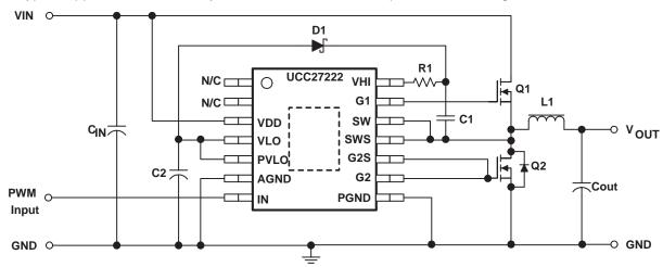
Figure 3. System Application: 8.5-V to 20-V Input
