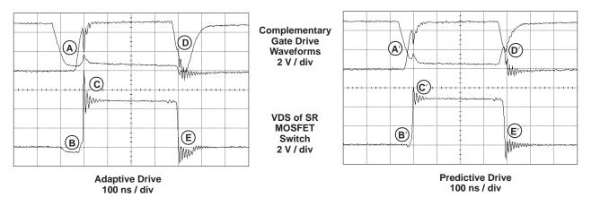
Figure 9. Adaptive vs. Predictive Switching Waveforms
