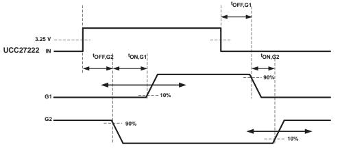
Figure 1. Predictive Gate Drive Timing Diagram
