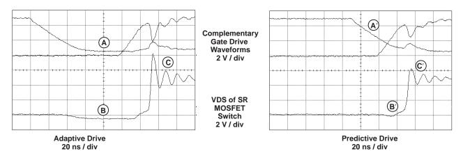
Figure 10. Close-Up: Turn-Off of Synchronous Rectifier Switch to Turn-On of Main Switch
