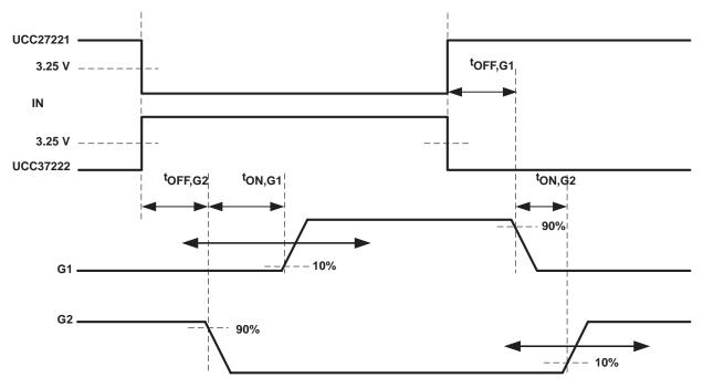
Figure 2. Predictive Gate Drive Timing Diagram
