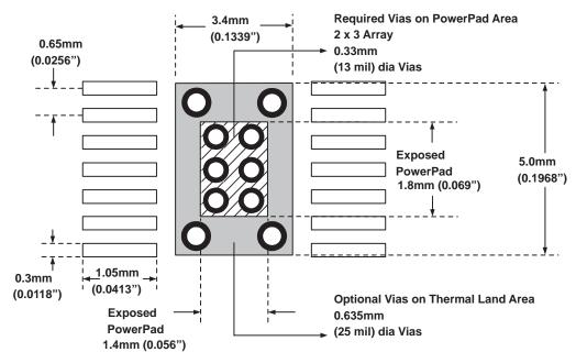
Figure 16. TSSOP-14PWP Package Outline and Minimum PowerPAD™ PCB Thermal Land
