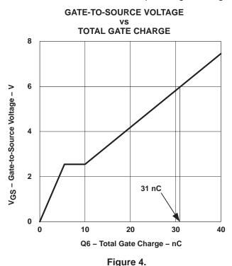
As shown in Figure 4, 31 nC of gate charge is required in order for Q1's gate to be charged to 6.0 V, relative to its source. The minimum bypass capacitor value can be found using the following calculation:
