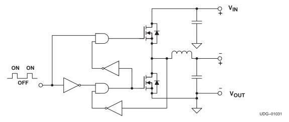
Figure 8. Adaptive Gate Drive Technique
