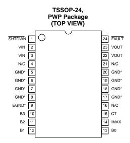
\*Pin 9 serves as lowest impedance to the electrical ground; other GND pins serve as heat sink/ground. These pins should be connected to large etch areas to help dissipate heat.
