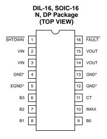
\*Pin 5 serves as lowest impedance to the electrical ground; Pins 4, 12, and 13 serve as heat sink/ground. These pins should be connected to large etch areas to help dissipate heat. For N Package, pins 4, 12, and 13 are N/C.
