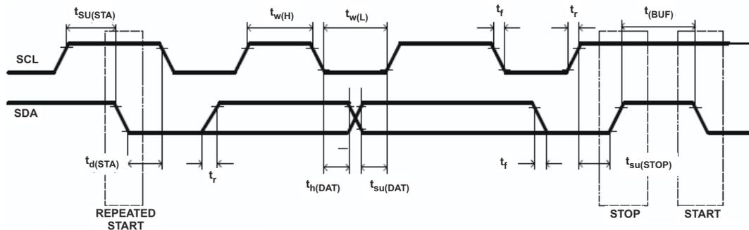
Figure 7-1. I<sup>2</sup>C Timing
