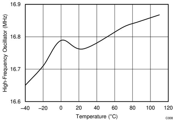
**Figure 7-6. High-Frequency Oscillator vs Temperature**
