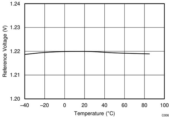
**Figure 7-4. Reference Voltage vs Temperature**
