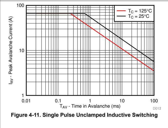
Figure 4-11. Single Pulse Unclamped Inductive Switching
