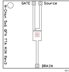
Max  $R_{\theta JA}$  = 125°C/W when mounted on minimum pad area of 2oz Cu.
