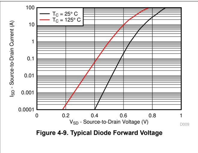
Figure 4-9. Typical Diode Forward Voltage
