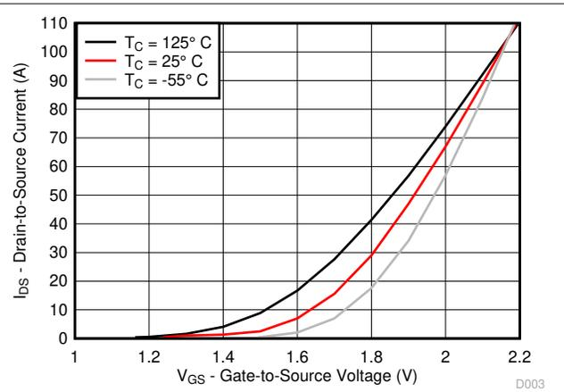
Figure 4-3. Transfer Characteristics
