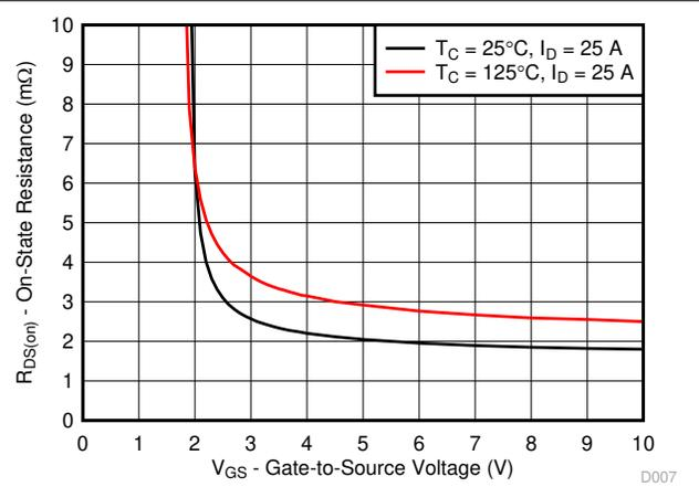
Figure 4-7. On Resistance vs Gate Voltage
