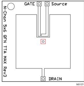
Max  $R_{\theta JA}$  = 50°C/W when mounted on 1in<sup>2</sup> of 2oz Cu.
