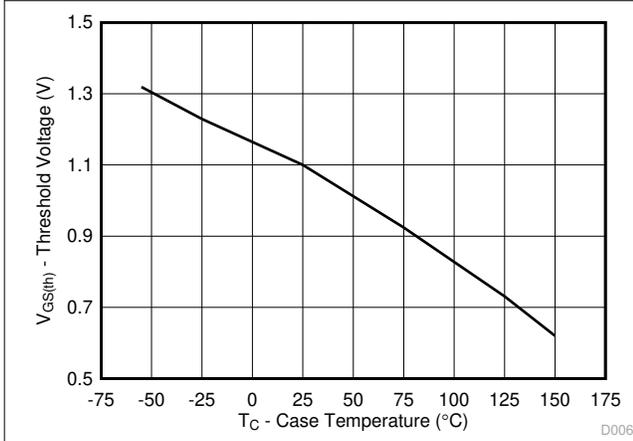
Figure 4-6. Threshold Voltage vs Temperature
