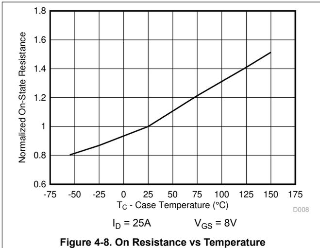
Figure 4-8. On Resistance vs Temperature
