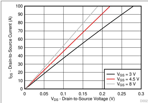
Figure 4-2. Saturation Characteristics
