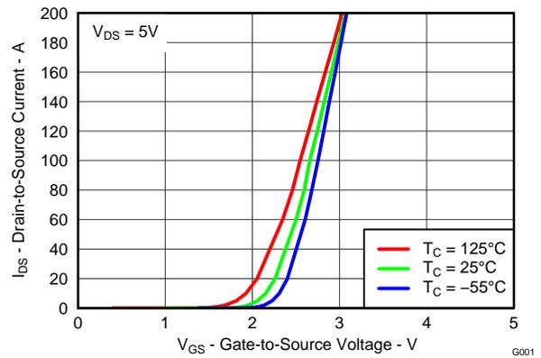
**Figure 3. Transfer Characteristics**
