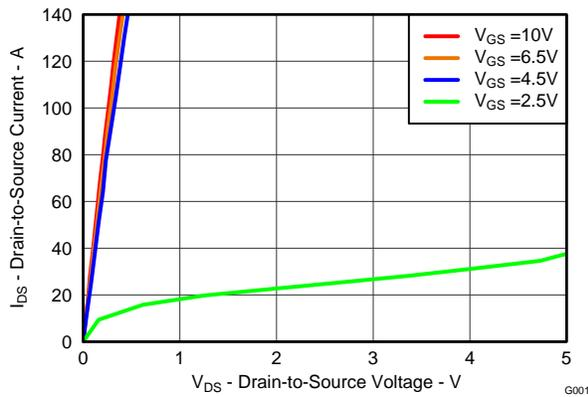
**Figure 2. Saturation Characteristics**
