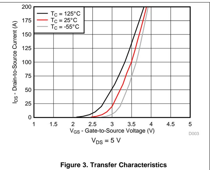
Figure 3. Transfer Characteristics
