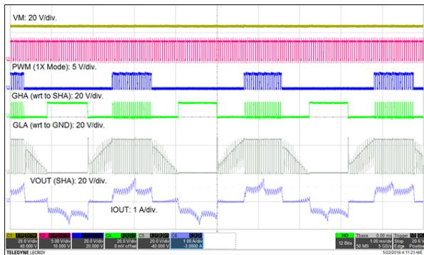
Figure 51. Motor Operation at 80% PWM Duty
