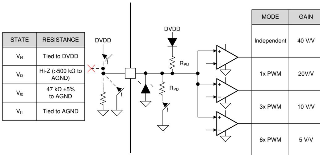
Figure 27. Four-Level Input Pin Structure (MODE and GAIN)
