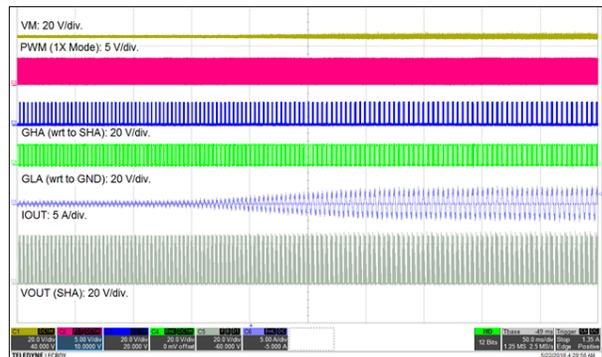
**Figure 56. Motor Performance at Load Change**
