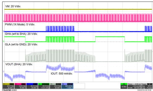
Figure 52. Motor Operation at 20% PWM Duty
