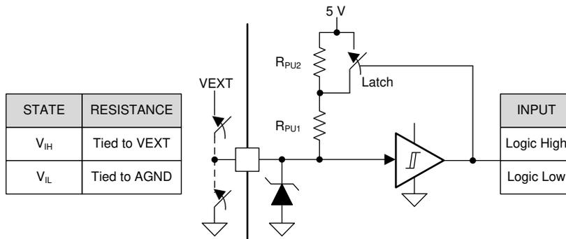
Figure 26. Logic-Level Input Pin Structure (ENABLE)
