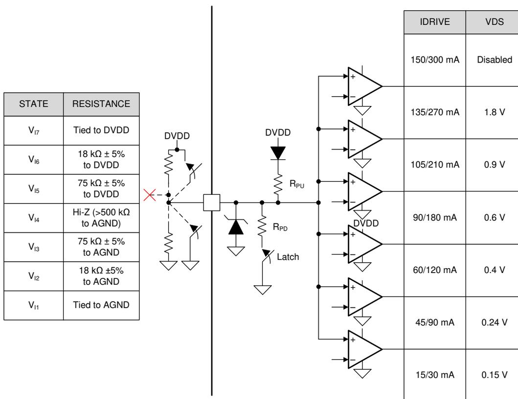
Figure 28. Seven-Level Input Pin Structure (IDRIVE and VDS)
