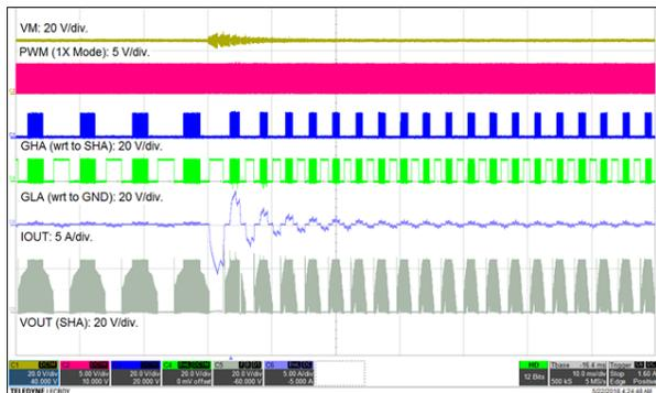
**Figure 55. Motor Performance at Speed Change**
