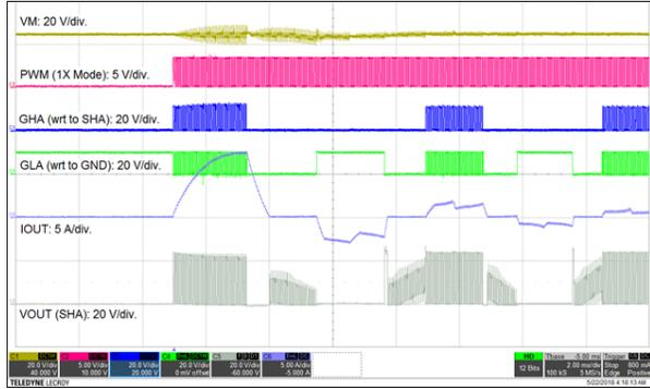
**Figure 53. Motor Starting With PWM Duty Change**
