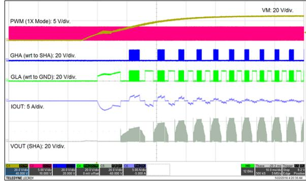
**Figure 54. Motor Starting With Supply Voltage Change**
