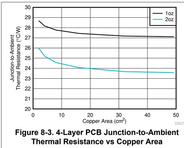
Figure 8-3. 4-Layer PCB Junction-to-Ambient Thermal Resistance vs Copper Area
