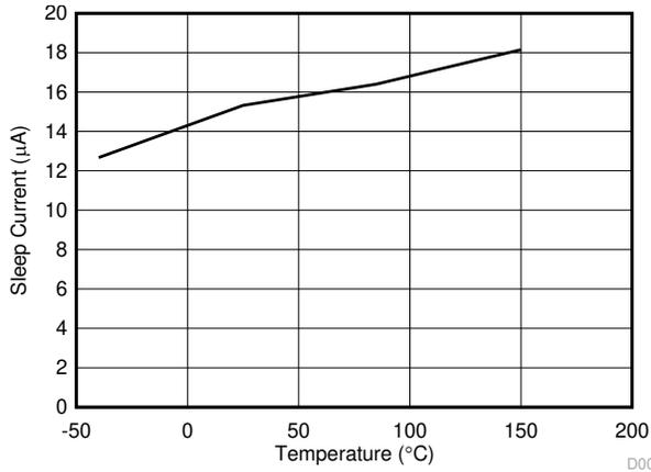
**Figure 6-4. Sleep Current (I<sub>VM(Q)</sub>) vs Temperature**
