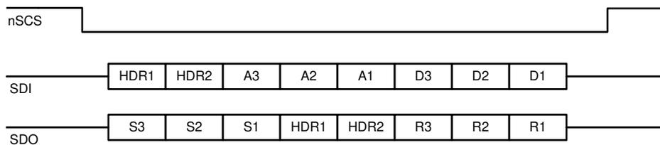
**Figure 7-19. SPI Data Sequence for Three DRV8873S-Q1 Devices**
