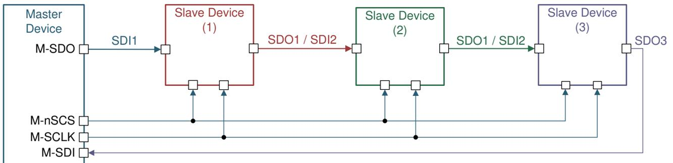
**Figure 7-17. Three DRV8873S-Q1 Devices Connected in Daisy Chain**
