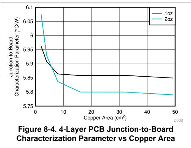
Figure 8-4. 4-Layer PCB Junction-to-Board Characterization Parameter vs Copper Area
