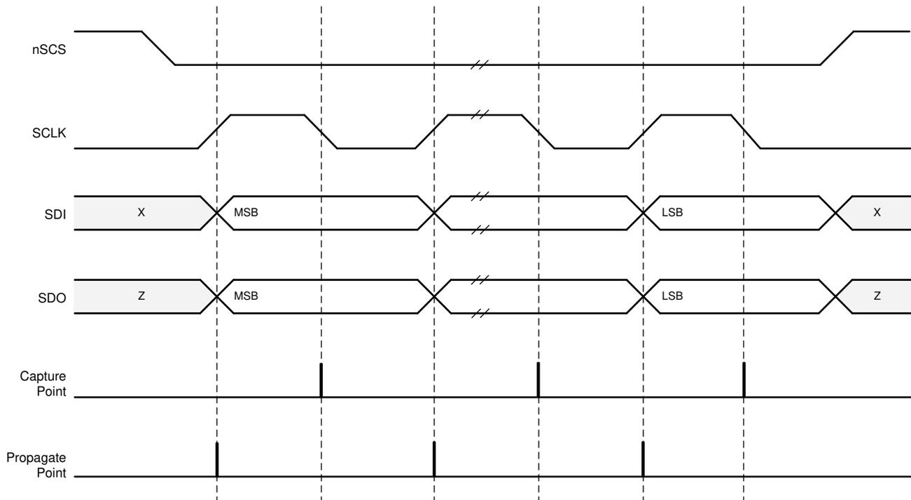
**Figure 7-22. SPI Transaction**
