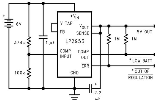
\* Connect to Logic or μP control inputs.
