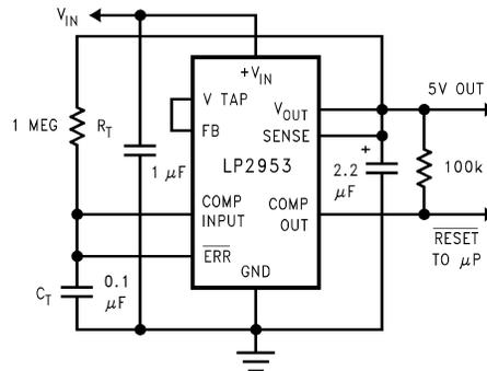
Figure 38. 5V Regulator with Timed Power-On Reset
