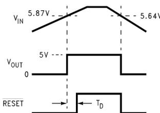
$T_d = (0.28) RC = 28 \text{ ms}$  for components shown.
