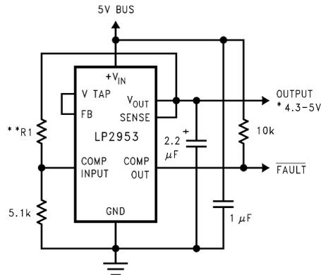
\* Output voltage equals +V<sub>IN</sub> minus dropout voltage, which varies with output current. Current limits at a maximum of 380 mA (typical).
